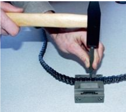
Layout13. Chain disassembly with the help of a mandrel and a hammer.
